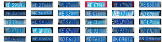
Fig. 6. Examples of license plates after tilt correction.
